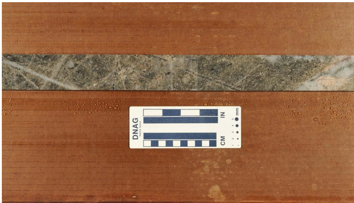
Photo 31. STD-06 core, 2863-65 ft, 2-ft-long unbroken stick of gray, andesite porphyry, biotite-K-spar alteration, 3 vol.% sulfide, and multitude of quartz±K-spar±sulfide±magnetite vein sets. All of the fractures have been rehealed by veins. Unbroken 5–10-ft-long sticks of core were commonly recovered from the bottom of STD-06 with 100% RQD (rock-quality designation).
