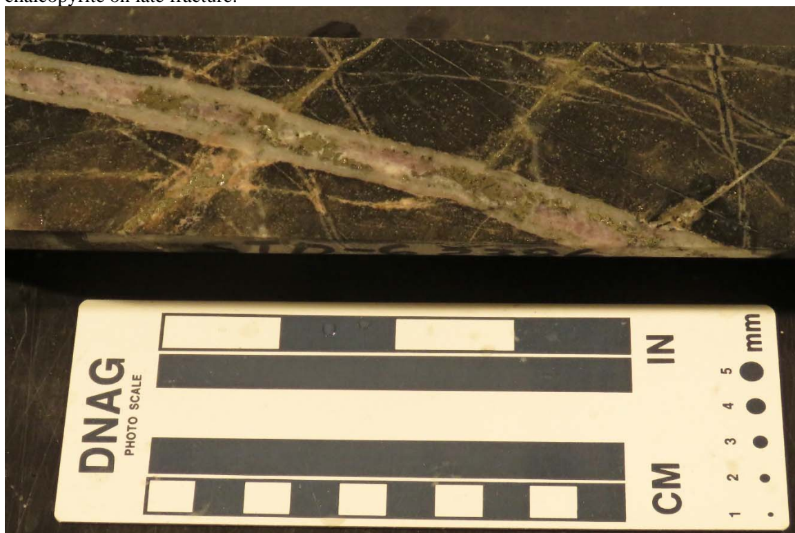
Photo 28. STD-06 core, 2386 ft, dark gray, andesite (?), strong biotite alteration, 2 vol.% sulfide, quartz-chlorite stockwork with bleached selvage cut by quartz-chalcopyrite vein cut by quartz-pyrite-molybdenite-anhydrite.
