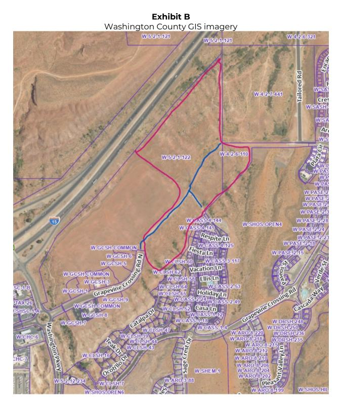
Crude outline of area needing to be graded shown roughly in red. Continuation of Grapevine Crossing North and secondary access road into the Casitas shown generally in blue.
