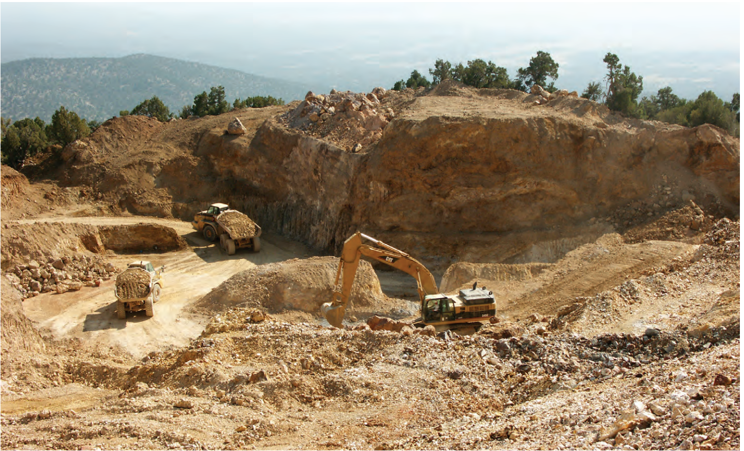
Photograph 19. Sandy Wash 4/Blawn Mountain kaolinite mine, just west of Blawn Mountain, looking west. This pit appears to be developed on a hydrothermal breccia pipe.
