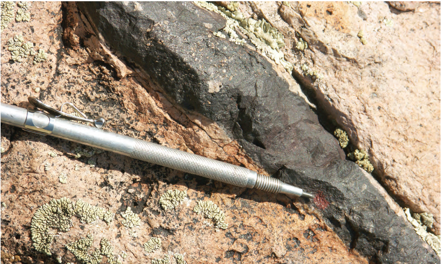
Photograph 7. Massive hematite vein (note red streak near tip of scriber) in Quartz-Alunite alteration on hill 7602 of Area B.
